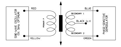
Note: the black wire is not used when connecting to RDP instrumentation. Ensure that this wire is insulated: it must not be allowed to short to other connections or screen.
