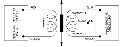
Note: the black wire is not used when connecting to RDP instrumentation. Ensure that this wire is insulated: it must not be allowed to short to other connections or screen.
