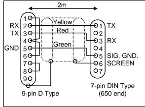
Fig. 3 Connections for RS232 lead.
