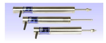
The ACT series displacement transducers form part of our industrial series of LVDTs. Because they use the LVDT principle they have a very long life as there is no electrical contact across the sensing element which means clean, reliable data. The ACT transducer gives an output proportional to the position of the armature assembly with respect to the body of the transducer. ACT series transducers are available in three versions as detailed below.
