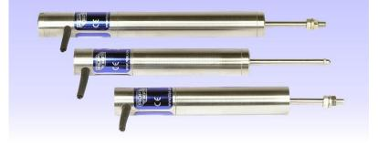
The ACT series displacement transducers form part of our industrial series of LVDTs. Because they use the LVDT principle they have a very long life as there is no electrical contact across the sensing element which means clean, reliable data. The ACT transducer gives an output proportional to the position of the armature assembly with respect to the body of the transducer. ACT series transducers are available in three versions as detailed below.
