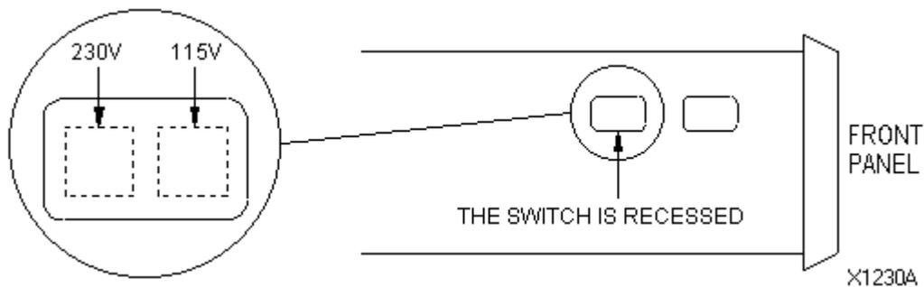
The E725 is fused internally but it is recommended that the unit be externally fused also. We suggest a fuse of a slightly lower rating to the internal fuse (details in Section 3.3) As this unit has no power switch, it is recommended that an external means of disconnection is fitted in a convenient location.
