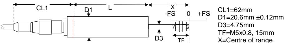
Our ACW captive guided displacement transducer has bearings to guide the armature inside the measurement sensor. Our ACW captive LVDTs are for position measurement applications where guidance may be poor and end bearings may be required.
