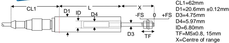
On our ACW unguided LVDTs the armature assembly is a separate component, to make a measurement the user must guide the armature inside the body without touching the sides. Our ACW unguided position measurement transducers are appropriate where external guidance is available and give truly non-contact operation
