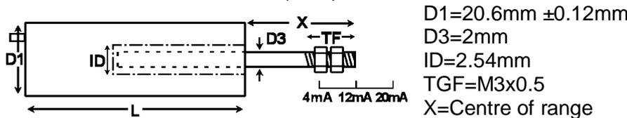
DCC025U to DCC0400U - Side (radial) exit cable
